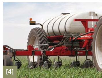
[1] Toolbar [2] Pumps [3] Coulters [4] Custom solution tank [5] Tires and Axles
