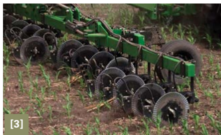
[1] Toolbar [2] Pumps [3] Coulters [4] Custom solution tank [5] Tires and Axles
