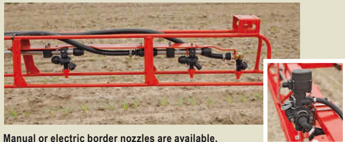
Manual or electric border nozzles are available.
