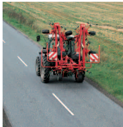
Despite a working width of 9m the Kverneland Taarup 8090 is very compact in transport, with a width of less than 3m.
