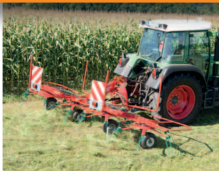
The angle for border tedding is set from the tractor cab.
