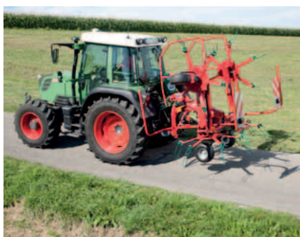
All tedders fold hydraulically from working to transport position.
