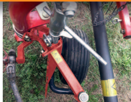
As an option the tedders can be equipped with a third wheel, to improve the ground contour followings.
