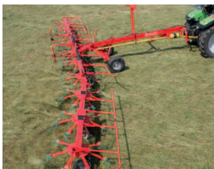
For border tedding the right outer arm is moved at the correct angle, to avoid loss of grass.
