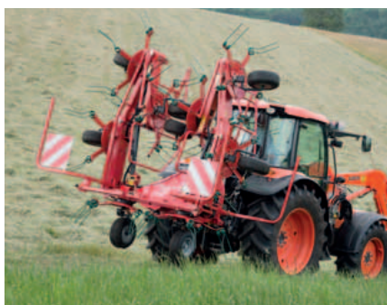
Despite its 8m working width, the Kverneland 8480 will fold to just under 3m, making it a very compact unit for transport
