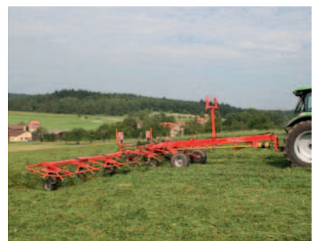
All operations are run hydraulically, including the unfolding process.
