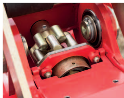
The two outer rotors are fitted with the new HexaLink finger clutch, a simple yet efficient drive system that permits these rotors to turn into a 180° position for transport.
