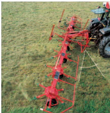
For border tedding the machine is swung at an angle to ensure no loss of grass, and all operations are carried out from the tractor cab.
