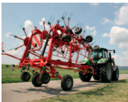
The outer rotors are fixed during transport and there is no load on the carrier frame.
