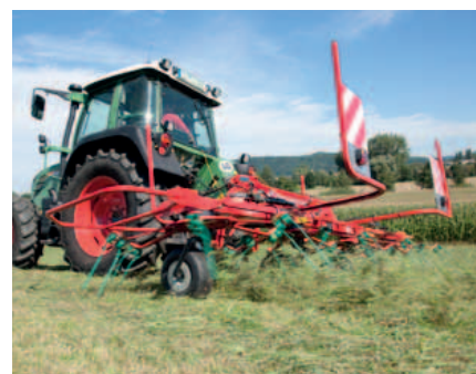
Kverneland Taarup 8452 with 5.2m working width.
