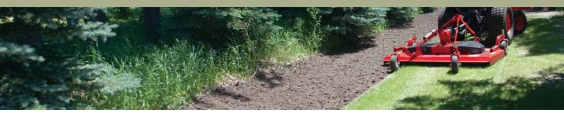
Model 430 - 4' (1.2 m) cutting width, 3-point hitch Category I For tractors 12 - 25 hp
