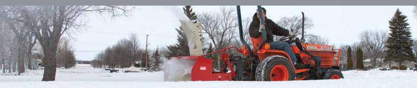
**Model 500** - 50" (1.3 m) cutting width For tractors 15 - 30 hp, 3-point hitch Category I
