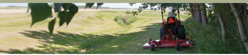
Model 555 - 5' (1.5 m) cutting width, 3-point hitch Category I For tractors 15 - 55 hp
