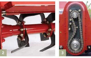
[1] The sideshift feature is available on the 45 Series and model 6572. [2] Flanges on all series are available with four tines. Six tines per flange are standard on the 65 Series. [3] Housed in a sealed oil bath, the chain tightener assembly is resistant to heat, dust, debris and moisture, which reduces maintenance and enhances the longevity of the chain and sprockets.
