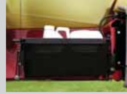
ChemLocker A ChemLocker can be fitted and holds chemical containers or bags.
