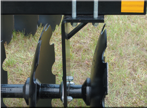
Bearing hangers reinforced with gussets
