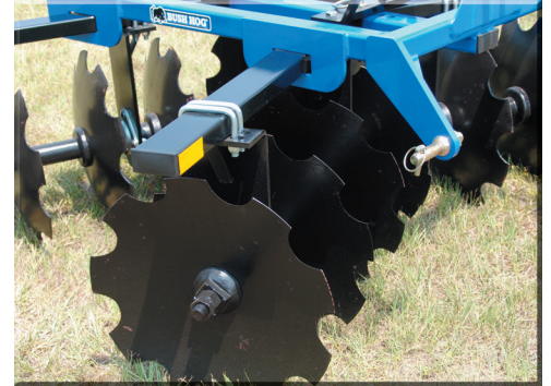
Notched discs for maximum cutting action
