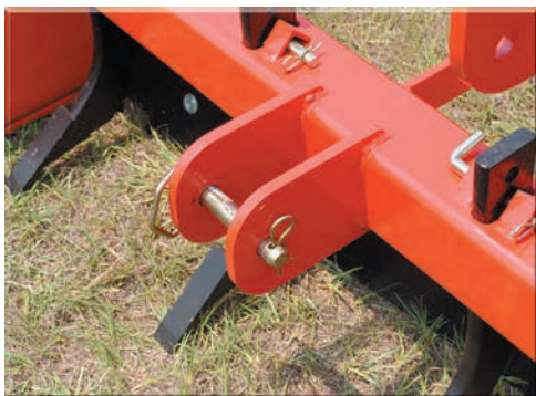
Scarifiers can rip soil up to 2-3/8" deep.
