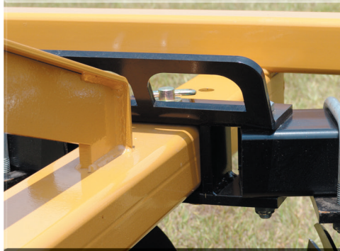
Easy-to-grasp handle for simple gang adjustment
