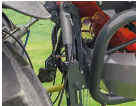
Border spreading with tramline cylinder - spreading towards the border from the last tramline
