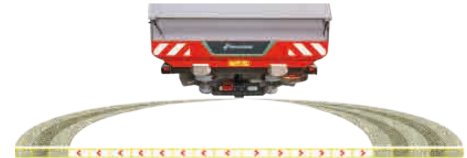
Switching off the sections outwards
