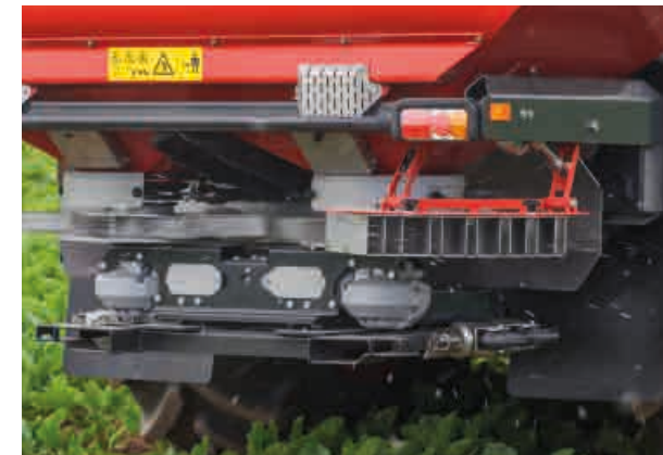
Border spreading - spreading to the border with the ExactLine
