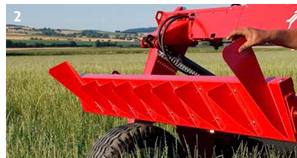
Changing from swathing to spreading is an easy operation. The rear plate is turned 180° (no tools required).
