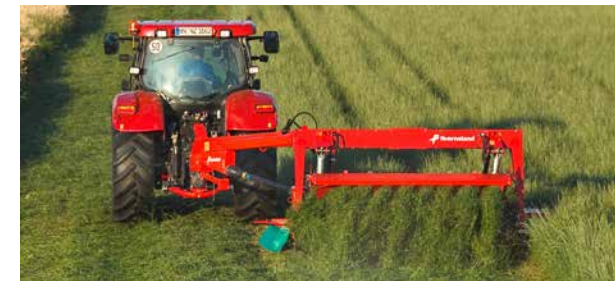
The crop is directed inwards, away from the unmown crop.
