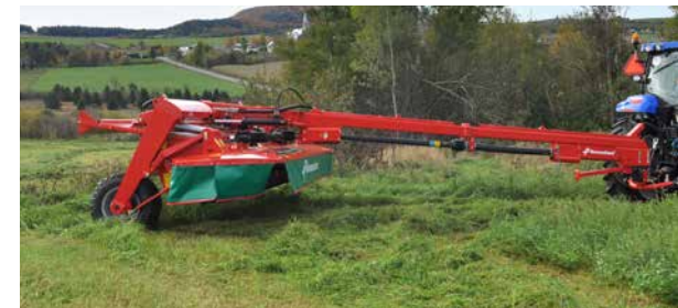
Centre pivot machines are easily manoeuvrable on headlands.
