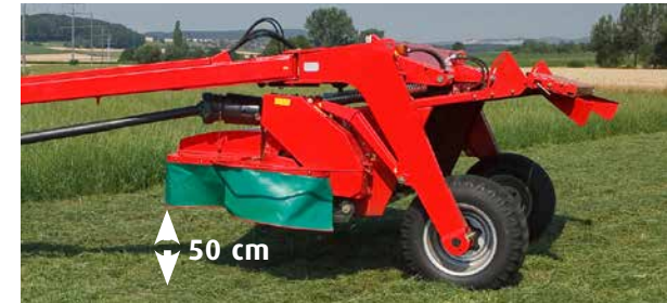
Clearance of 50 cm due to the design of the trolley.
