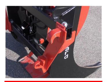
The grip claw comes without suspension. Fransgard can deliver EURO or SMS brackets, which can be bolted on.
