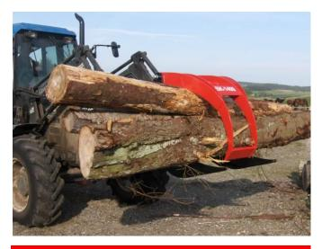
The upper arm securely holds the timber against the long forks, even if the middle grip is not right
