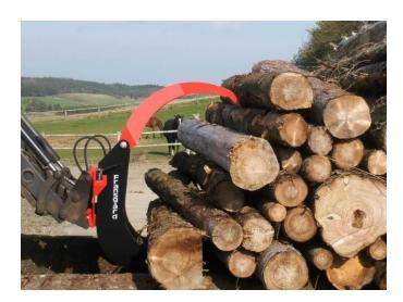
The large opening height of the upper arm and long forks allows for large volumes of timber to be grapped.
