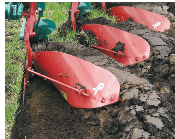
furrow profile body No. 28 working depth: 26 cm, bottom: 30 cm, width 73 cm
