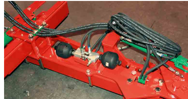
As standard, 2 accumulators are fitted to the BE plough for safe steering
