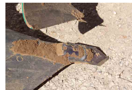
Soil flow protects other parts.
