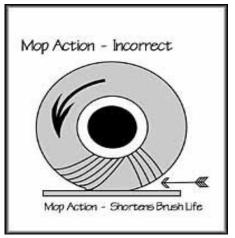
A broom sweeps with the tips of its bristles. When too much down pressure is applied, the broom is working with the sides of the bristles limiting the flicking action, the effectiveness of the sweeper and shortening the broom life.
