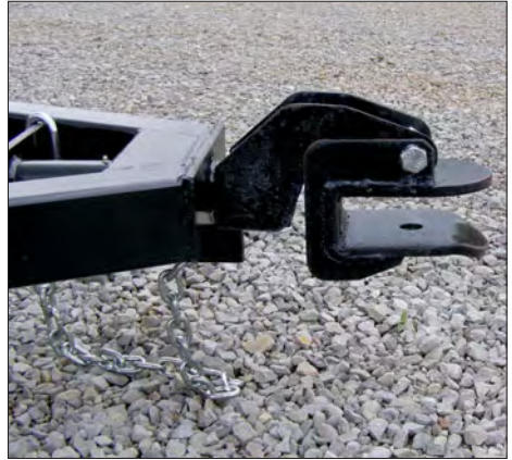
FLAT SWIVEL HITCH Greatly reduces drawbar wear
