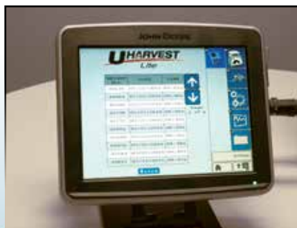
UHarvest Lite scale package displays up to 400 unloading events showing weight, date and time
