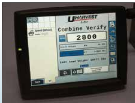
Combine Verify feature for easy combine yield monitor calibration
