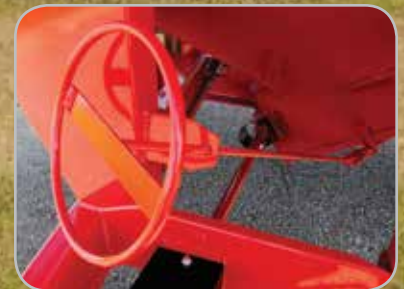
Wheel-operated cleanout door
