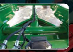
The load-equalizing torsion-bar rear axle design, coupled with the rocking-arm bolster, keep Grain Train wagons level and stable during loading and transport, and quiet when empty, even over the bumpiest gravel roads.
