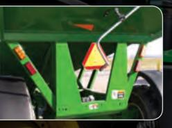
All models feature DOT-approved LED side-marker lights and red flashing amber taillights for enhanced durability and greatest light with lowest voltage use. Reflective striping, SMV emblem and transport chain are also standard for greater transport safety.
