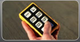
Optional wireless remote control for unloading door on Q-series models for ultimate unloading convenience, even from the tractor cab. Remote also includes open/close feature for electric-operated tarps.
