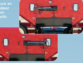
The 757Q, 657Q and 557Q models come standard with an exclusive **pushbutton-controlled unloading door** with front and rear switches for ultimate unloading convenience.
