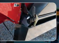
Gas-strut lift-assist unloading chute with spring-loaded locking mechanism for effortless use. Door height can be adjusted from 15" to 18" with center deflector. Optional right-side unloading.
