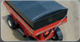
Rollover, 18-ounce canvas Weatherguard tarp for protecting load contents; automatic self-locking design keeps tarp securely in place during transport. Optional electric open/close.
