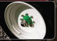
Oil-bath hub housing for greater durability and easier maintenance.
