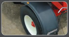
Molded plastic fenders protect finish and include LED side marker lights for added visibility.
