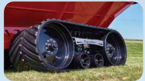
Equalizer™ tracks for optimum flotation
