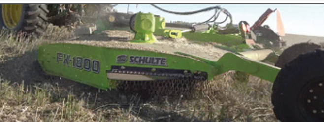
Outboard blade rotation keeps material from balling up under the deck
