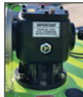
Oil level site glass on gearboxes
