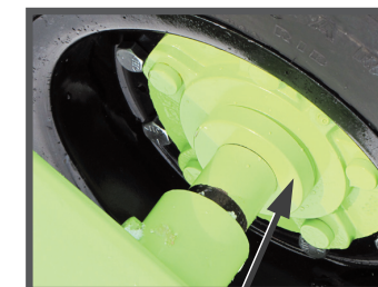
Metal seal guards on 517 hubs
