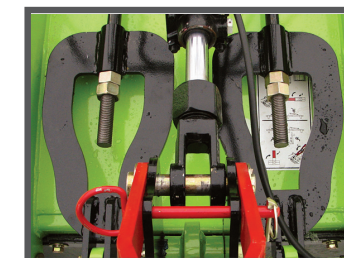
Dual levelling rods with floating hitch
