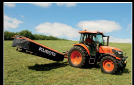
Lift on headlands via a hydraulic cylinder – no use of the 3 pt hitch is needed.
