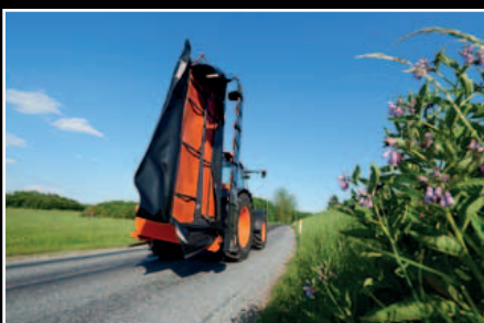
For transport the machine is folded hydraulically from the tractor cab to the vertical transport position well behind the tractor, ensuring a stable and steady transport.
