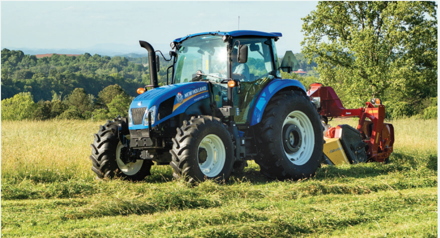
12x12 speeds with 4WD front axle and 18R34 tires
