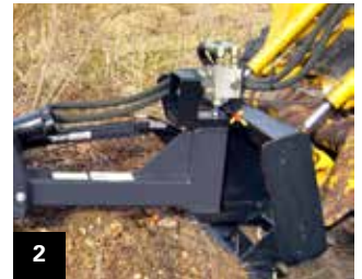
[2] Manual tilt adjustment up to 15 degrees.
