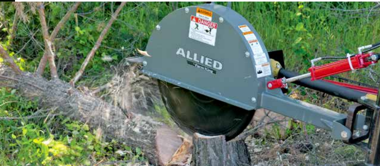
[1] Large 26 and 36 inch cutting wheel diameter.
