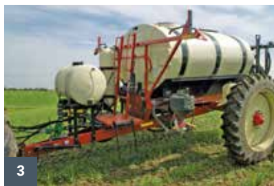
[1] Boom suspension [2] Lattice-style boom [3] Frame [4] Custom solution tank [5] Tires and axles
