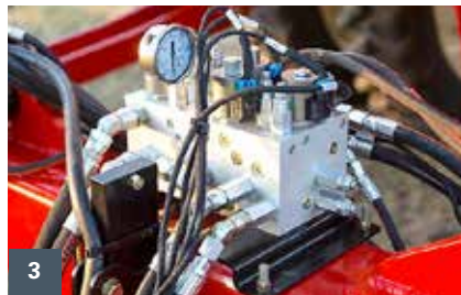
[1] 175" wheelbase [2] A wide stance, high clearance, parallel lift linkage [3] Hydraulic valve block [4] Visual flow monitor system [5] Toolbar proximity sensors
