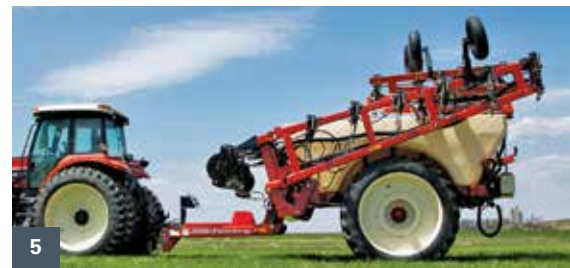
[1] Folded for transport [2] Rotational lift toolbar [3] Asymmetrical tank design [4] Tires and axles [5] Transport position
