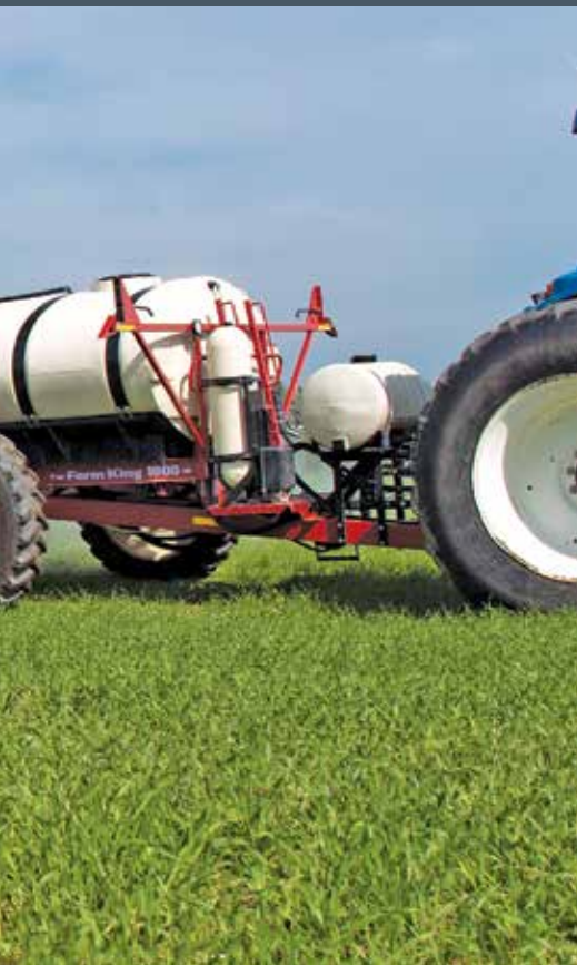
[1] Boom suspension [2] Lattice-style boom [3] Frame [4] Custom solution tank [5] Tires and axles
