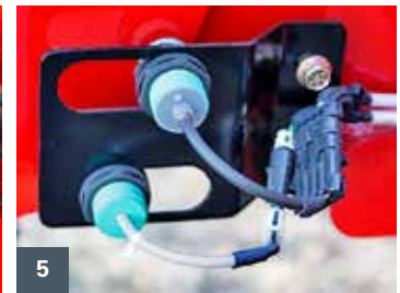
[1] 175" wheelbase [2] A wide stance, high clearance, parallel lift linkage [3] Hydraulic valve block [4] Visual flow monitor system [5] Toolbar proximity sensors
