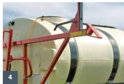
[1] Boom suspension [2] Lattice-style boom [3] Frame [4] Custom solution tank [5] Tires and axles
