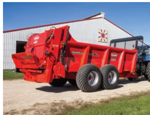
All beater modules are easily removable for maintenance, stockpiling or switching of modules.
