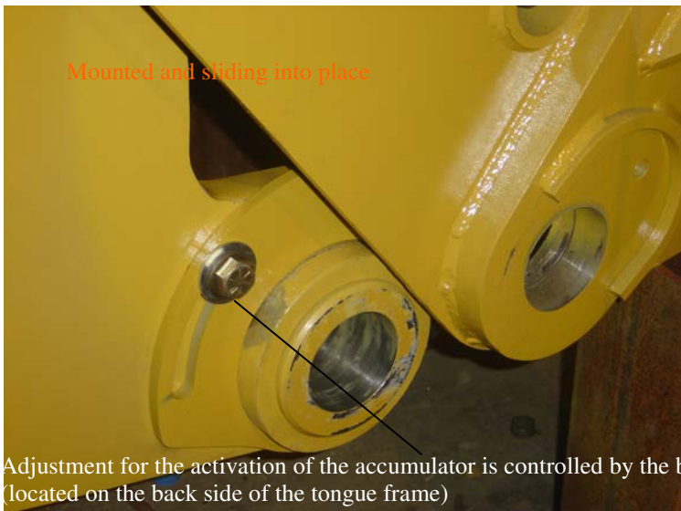
Valve installed and the adjustment bolt shown
