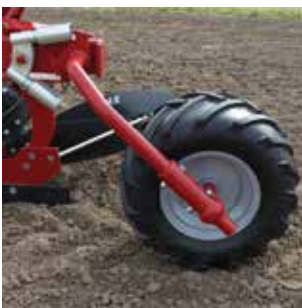
Tractor patterned tire for types R, MR, HR (4). 26*12,00-12
