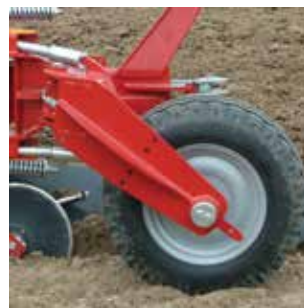
Rear mounted combiwheel for type HR and XR. 10.5/65-16 / 340/55-16
