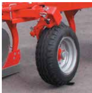
Sidemounted combiwheel for type HR. 10.5/65-16.
