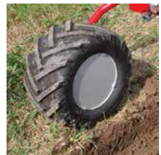
Rim side tractor patterned tire. Counteract soil covering.
