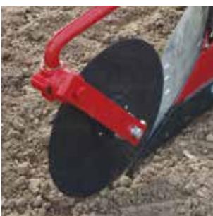
Disc coulters are available in plain or grooved, flexible or rigid.
