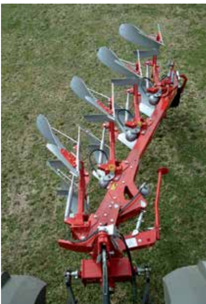
A parallelogram automatically adjusts the alignment.
