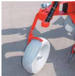
Land wheel, steel, for types R and MR. 500 x 160 mm.
