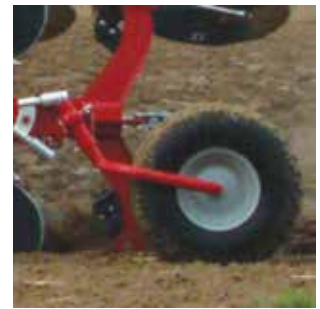
Combiwheel for types R and MR. 10.0/80-12.
