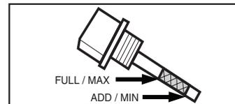
Be sure the machine is level when checking the oil level. (Refer to the engines operating manual for seasonal grades). We recommend that the oil be changed after the first 5 hours of use, then once every 50 hours.
