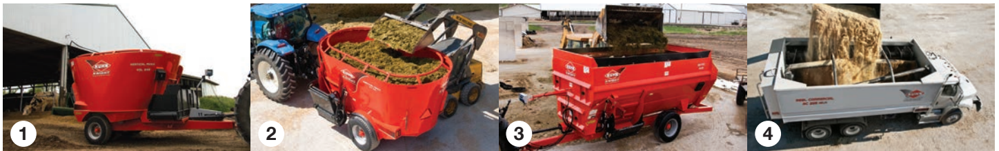
1. Single-auger vertical TMR mixers / 2. Twin-auger vertical TMR mixers / 3. 4-auger horizontal TMR mixers / 4. Reel TMR mixers
