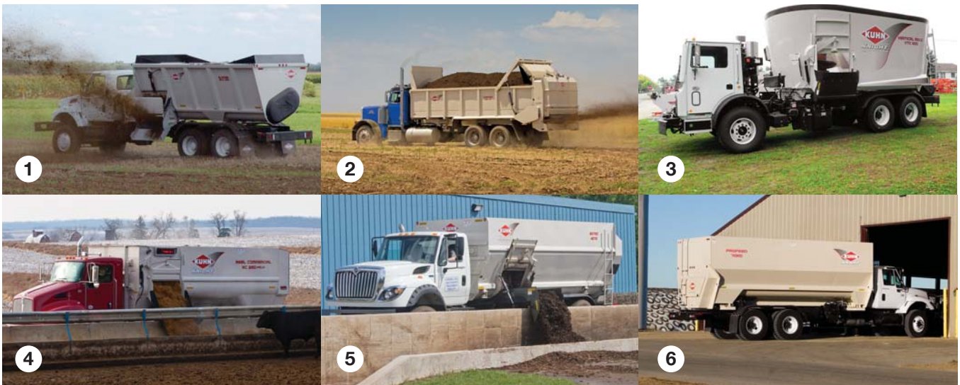
1. Side-Discharge Spreaders – 2. Apron Box Spreaders – 3. Vertical Twin-Auger Mixers – 4. Reel Mixers – 5. 4-Auger Mixers – 6. Delivery Boxes
