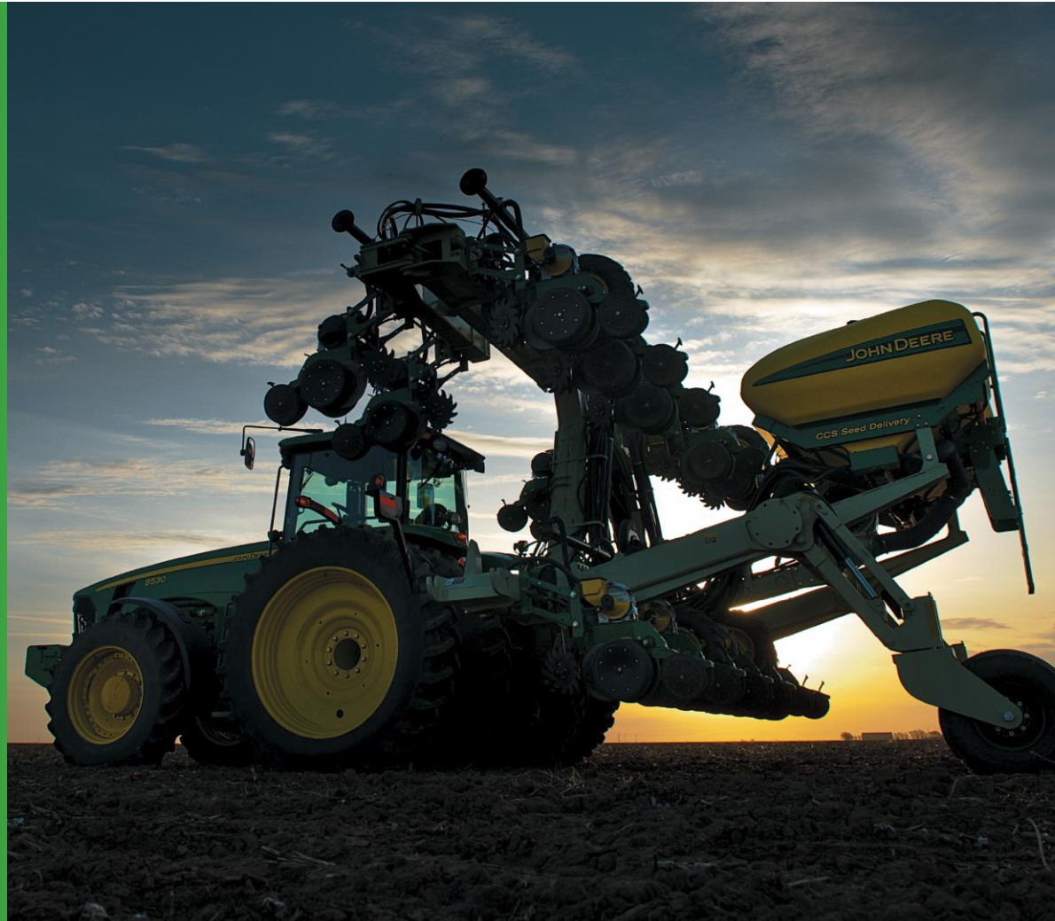
The Custom-built, 12-row integral planter from John Deere and Orthman® Manufacturing is for the producer who wants a 12-row stack-fold planter with the Central Commodity System.
