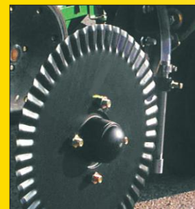
Unit-mounted single-disk liquid-fertilizer injection system openers use a single, 50-wave coulter to penetrate tough seedbeds. The liquid fertilizer is injected into the soil directly behind the coulter. For use with select planter models.
