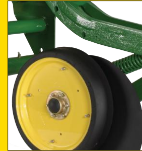
The single-disk fertilizer opener works well for no-till, double-crop, and reduced-till fields, plus firm-soil conventional seedbeds. A 13-inch rubber wheel gauges depth and minimizes soil disruption. A cast spout keeps soil from flowing into the furrow before fertilizer is delivered.
