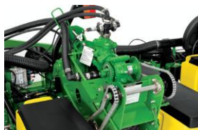
The liquid fertilizer system works with both fixed-rate (shown at left) and variable-rate pump options. The system can be ordered with openers, or without for in-furrow application.
