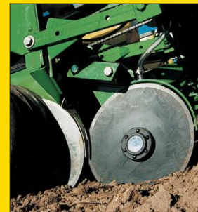
Unit-mounted double-disk openers for liquid fertilizer disturb less soil. Fertilizer can be placed even with seed depth or one inch below. The opener can be positioned up to 2 1/4 inches off the row. Ideal for conventional, reduced-till, and light no-till fields.
