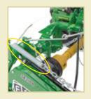
The SB31 Series are equipped with an additional spring *(highlighted)* to reduce the pressure on the cutter bar while working.
