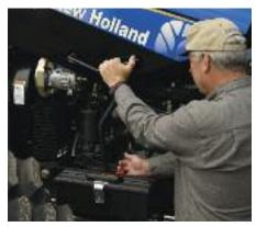
Pull this lever and the entire hood flips up for complete engine access.
