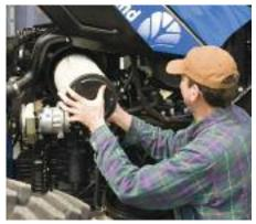
The engine air filter is accessible from ground level. Easy, spin-off wing nuts make cleaning or replacement a breeze.
