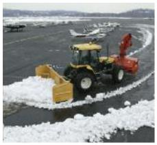
You get double-duty with the Bidirectional  $^{\text{TM}}$  tractor. A PTO, three-point hitch, and drawbar at each end let you push and pull implements at the same time, doubling your productivity.
