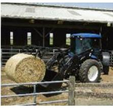
Articulated steering lets you make sharp turns and maneuver in tight areas a typical tractor can't. If one end of the tractor fits, the other end will, too.
