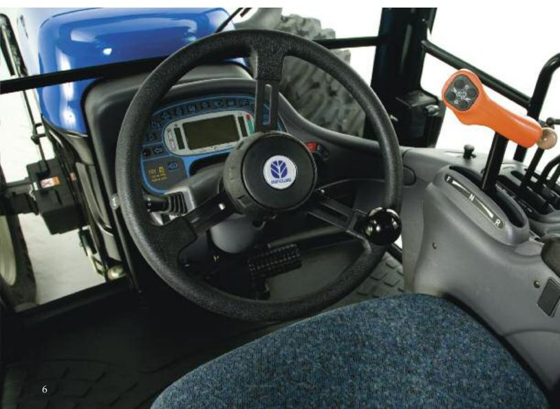
and remain that way regardless of which direction you're facing. Whether the console is facing the cab end or the engine end, it can be offset 15 degrees as a single unit for added comfort when looking back. And, since the cab has two doors, you can enter or exit the cab from either side, depending on the position of the Turnabout console.
