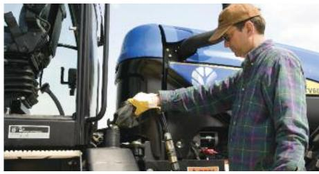
The high-capacity 55-gallon (total capacity) fuel tanks are located in front of the cab steps and can be reached conveniently from the ground and filled from either side.
