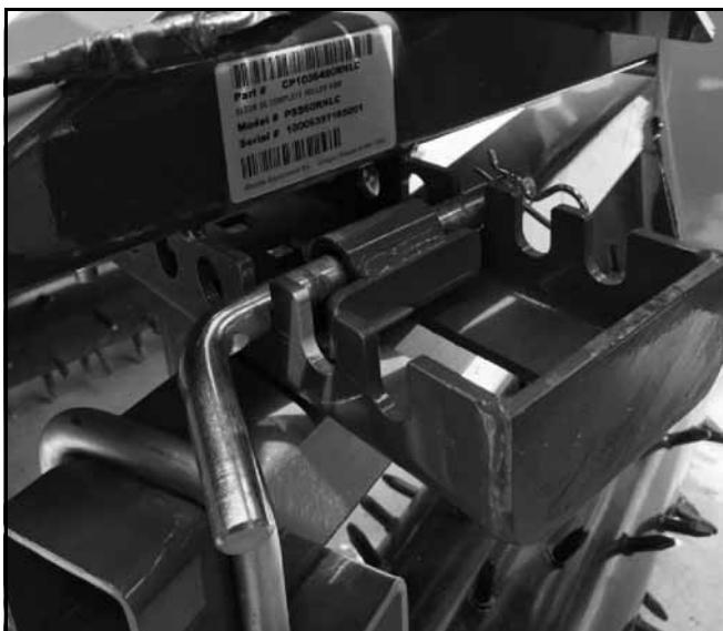
Figure 14. Bent Pin Installation
