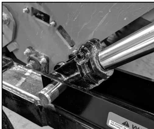
Figure 35. Cylinder Rod End Installed
