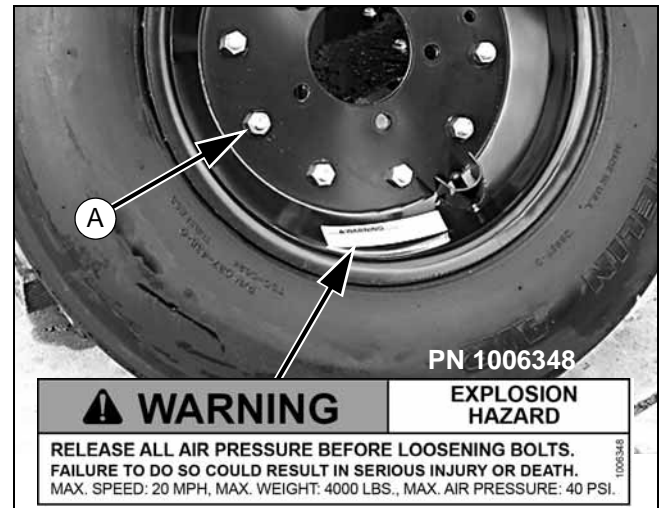
Figure 34. Split Rim Tire Servicing
