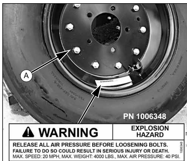
Figure 21. Split Rim Tire Servicing
