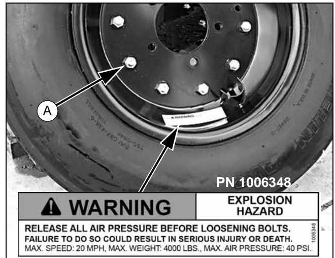
Figure 9. Split Rim Tire Servicing
