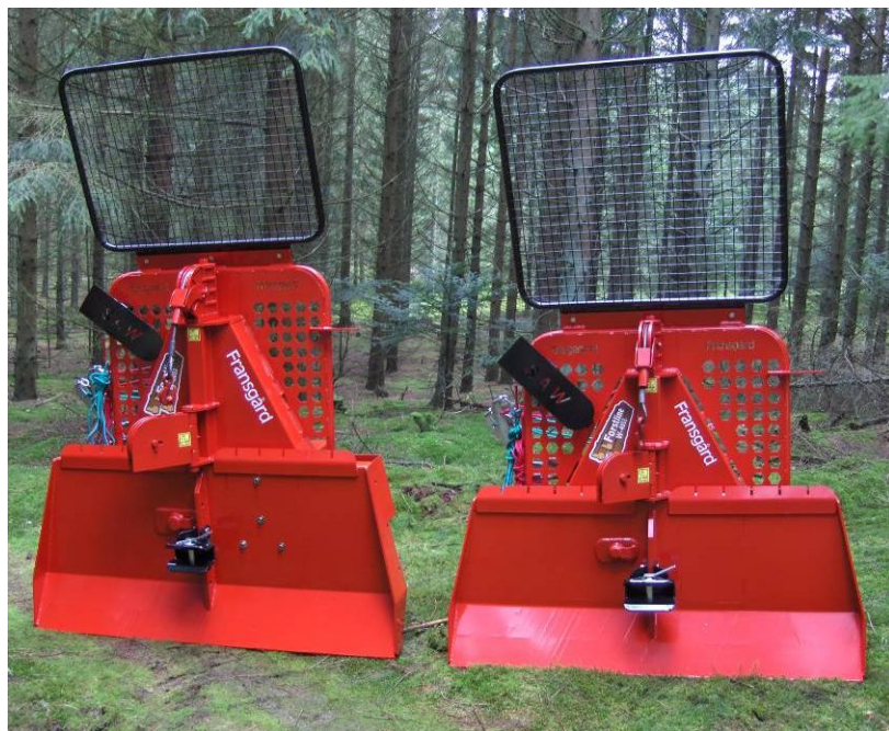
The unique design of the winch includes the smallest detail. The sturdy frame construction is made from special steel. A solid, wide blade/butt plate and lower pulley are standard. Chainsaw holder and trailer attachment are optional.
