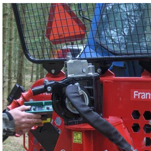
W-6011-EH with optional hydraulic device for unwinding wire rope, relieves the heavy work of pulling the wire out.
