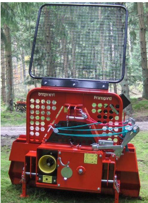
Several protection screens and a “noiseless” chain tightener ensures a safe and good working environment for the user.
