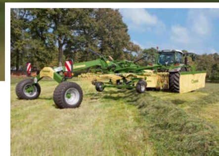
Swadro TS 680 Twin Work width: 6.80 m (2 rotors of 3.80 m each)
