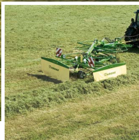
Forming one double swath Raking 12.40 m into one double swath
