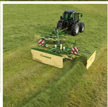
Forming one single swath Raking 6.20 m into one swath
