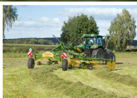
Swadro TS 620 Twin Work width: 6.20 m (2 rotors of 3.46 m each)
