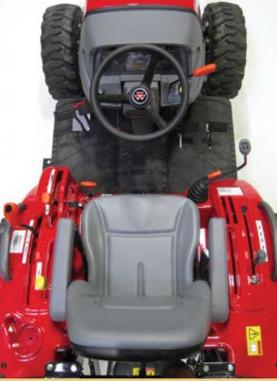
Separate forward and reverse pedals on the uncluttered platform are easy to operate and offer infinite ground speeds. Increasing engine speed is as simple as pushing the pedal. We also moved the brake pedals to the left side of the platform for ease in using the steering brakes.
