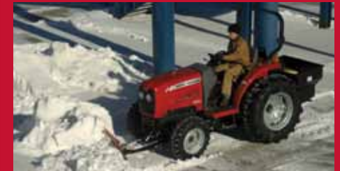
I405/I545/I550 Front Blade I405 Width: 66" (1,676 mm), I545 Width: 72" (1,829 mm), I550 Width: 84" (2,134 mm)
