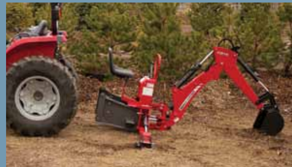
Step 3 Lower stabilizers to steady backhoe while storing. Shut off tractor and disconnect hydraulic hoses.
