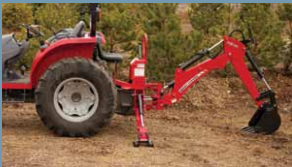
Step 1 Lower stabilizers slightly off the ground. Extend boom to raise tractor slightly and remove mounting pins.
