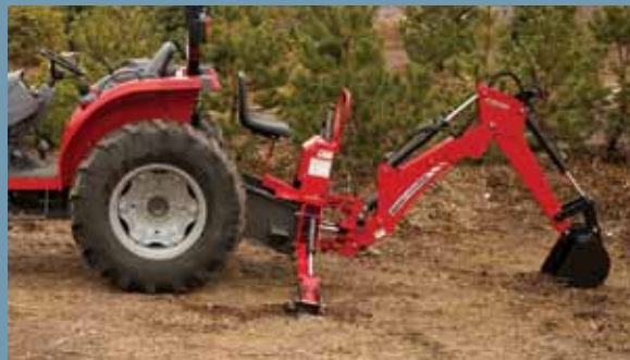
Step 2 Use boom to let backhoe roll back and out of the cradle.
