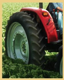
Each model comes equipped with 50-inch tires, providing a generous 22-inch ground clearance.
